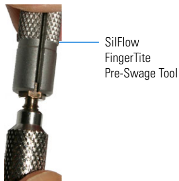
Figure 12. Swaging the Ferrule Using the SilFlow FingerTite Tool
