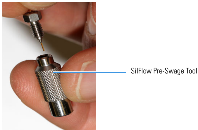
Figure 11. Inserting the Column and Ferrule into the SilFlow Pre-Swage Tool
