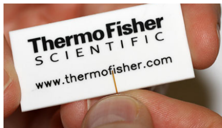
Figure 10. Cutting the Tubing with the Scoring Wafer
